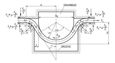
angle of wrap \*insert A\* is recorded for draw-bead and the groove. The \*insert A\* angle of wrap is derived from the draw-bead geometry and the depth of the draw-bead. Friction is taken into account using the relationship valid for rope friction. The bending radii are in all cases the radii of the draw-bead and the groove.
