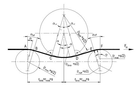
The principle of the mathematical model used for the calculation of bend radii
