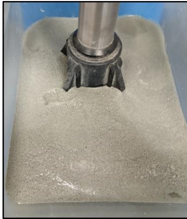
Figure 2: Foam layer at the pulp-air interface (no aeration or frother addition).
