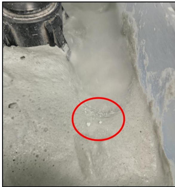
Figure 5. 3: Dry aggregates remaining on the pulp surface during the conditioning stage.
