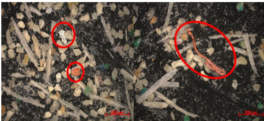
Figure 5. 4: Microscopic analysis of dry aggregates showing entrapment of metallic particles.
