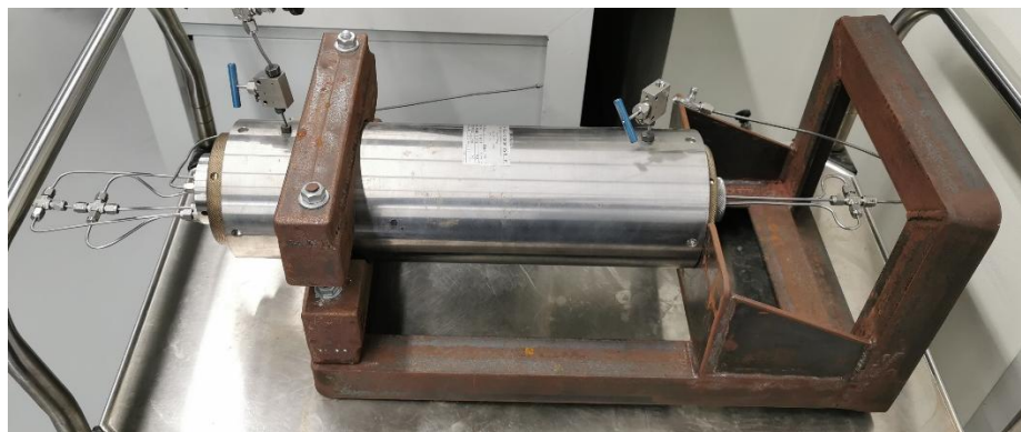
Figure 2 The novel core holder
