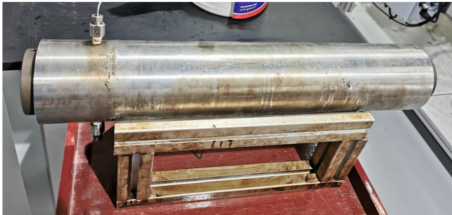
Figure 1 Core holder used for single and dual-core flooding experiments
