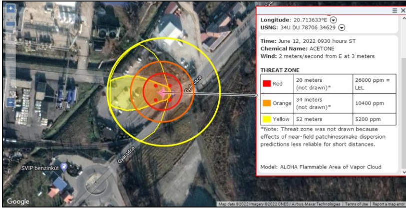
Figure 4: Depiction of LEL 20%, LEL 40% and LEL concentrations resulting from the evaporation of a large liquid surface area with an air flow of 2 m/s (edited by the author)
