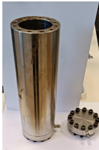
Figure 23. The cell used for CO 2 flooding (Recorded by the author)
