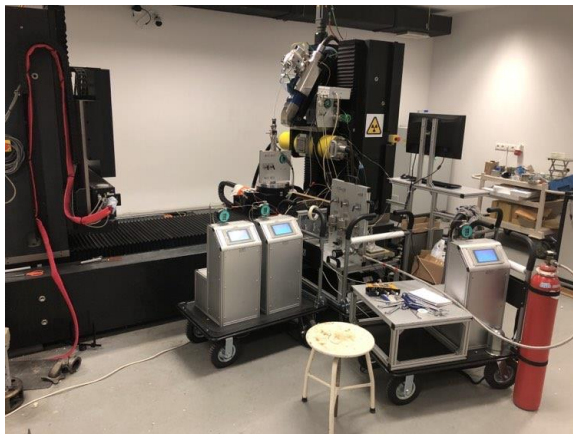
Figure 37. Network diagram and photos of the displacement device which was coordinated with the mCT device (Recorded by TOMOGEO Ltd.)
