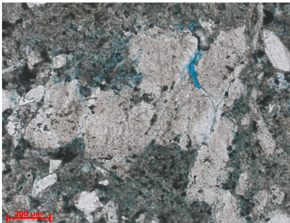
Figure 130. Quartz (Q) grains and muscovite (Ms) sheets with increased intergranular space (blue). Bottom: enlarged image of the polycrystalline quartz stack shown in the image above, Left 1N, right XN (source: UoM)
