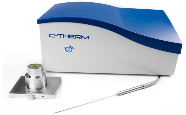
Figure 30. Thermal conductivity analyser instrument (C-Therm TCi)
