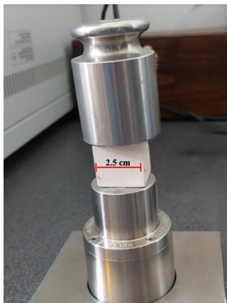
Figure 36. Geopolymer binder thermal conductivity sample.
