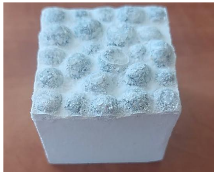
Figure 34. Flotation of foam glass aggregate in the geopolymer binder.
