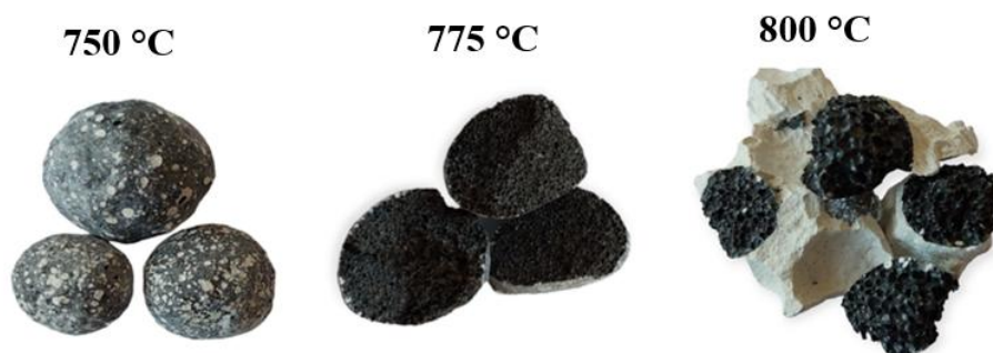
Figure 77. The FGA fracture shape after the compressive test for LWGP.
