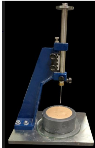
Figure 37. Vicat apparatus for the measurement of the setting time of the geopolymer binder.
