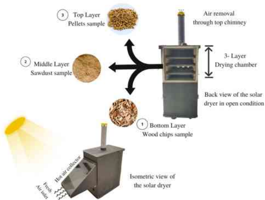
Figure 11. Experimental setup of the solar dryer for the investigations.
