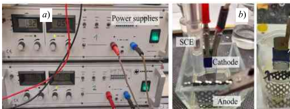
Fig. 6.1 Galvanostatic power supplies (a) and the experimental cell (b).
