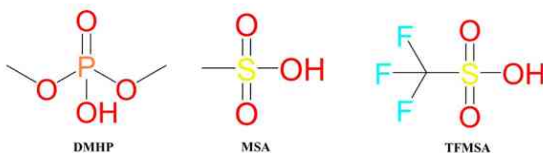
Figure 46. Chemical structures of the studied catalysts: dimethyl hydrogen phosphate (DMHP), methanesulfonic acid (MSA), and trifluoromethanesulfonic acid (TFMSA).
