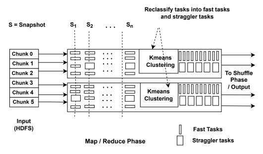
Figure 4.4: Structure of Task Performance Monitoring Algorithm
