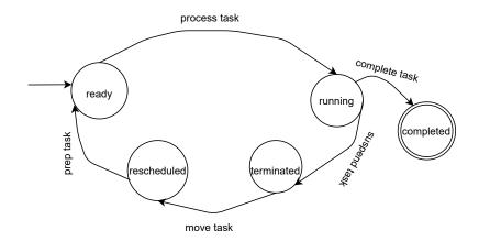
Figure 4.3: Rescheduling of Tasks State Diagram
