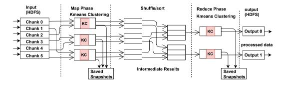
Figure 4.5: Structure of Our Approach Implementation with Kmeans Clustering
