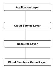
Figure 2.2: General Architecture of a Cloud Simulator
