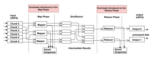
Figure 4.8: Overheads Introduced by Our Approach on MapReduce
