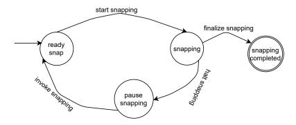
Figure 4.2: Snapshot Capturing State Diagram
