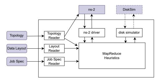
Figure 3.2: Mperf Structure [164]
