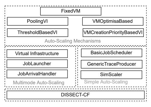
Figure 5.1: Architectural view of Auto-Scaling Mechanisms on DISSECT-CF
