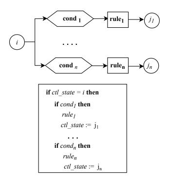
Figure 2.3: Control state ASMs
