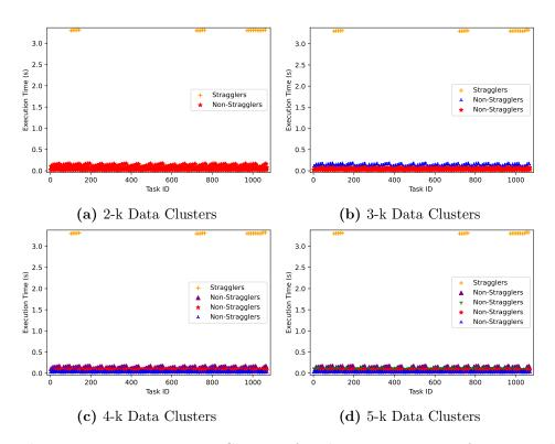
Figure 4.14: Kmeans Data Clusters of Tasks Execution times from 20 Nodes by 8 Cores Data Centre with Disruption
