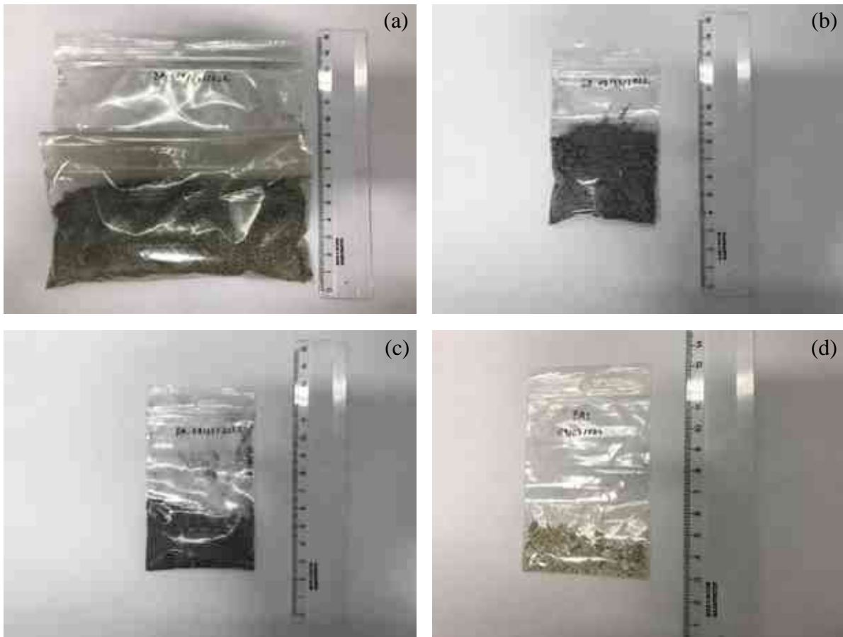
Figure 4.7. An example of ash samples collected from 20-kW contaminated biomass combustion experiment C20. (a) Bottom ash, (b) After exchanger ash, (c) Deposited ash, (d) Fly ash.
