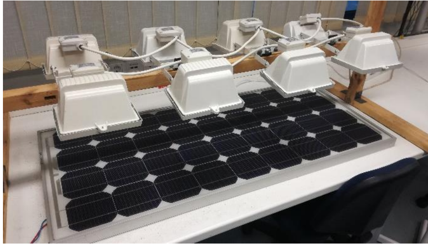
Figure 2. The solar panel illuminated by the solar simulator.
