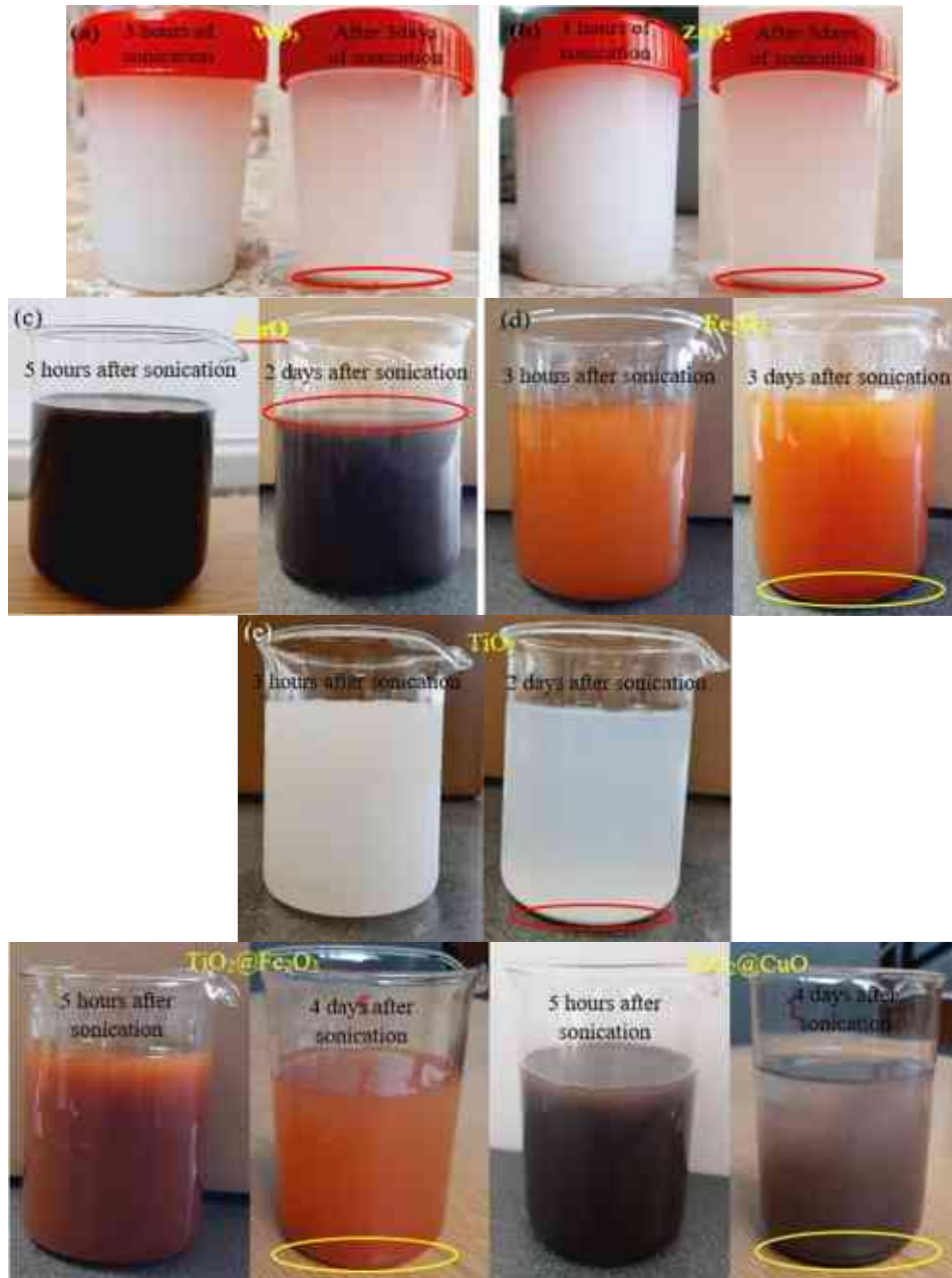
Figure 2.9: Stability of preparation of nanofluids (a) \text{WO}_3/\text{DI} water, (b) \text{ZrO}_2/\text{DI} water, (c) \text{CuO}/\text{DI} water, (d) \text{Fe}_2\text{O}_3/\text{DI} water, (e) \text{TiO}_2/\text{DI} water, (f) \text{TiO}_2\text{-Fe}_2\text{O}_3/\text{DI} water, (g) \text{TiO}_2\text{-CuO}/\text{DI} water
