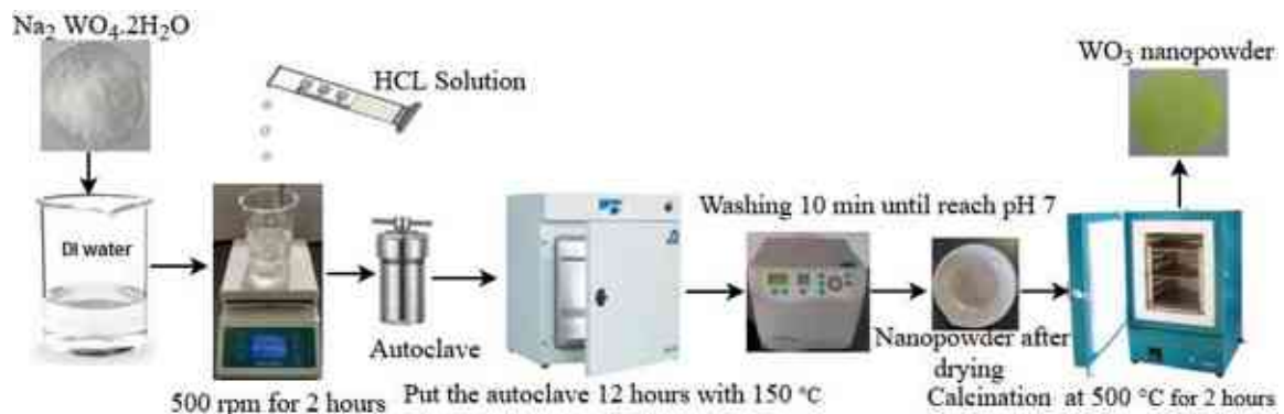
Figure A.1: Schematic of the synthesis process of WO_3 nanopowder by hydrothermal method
