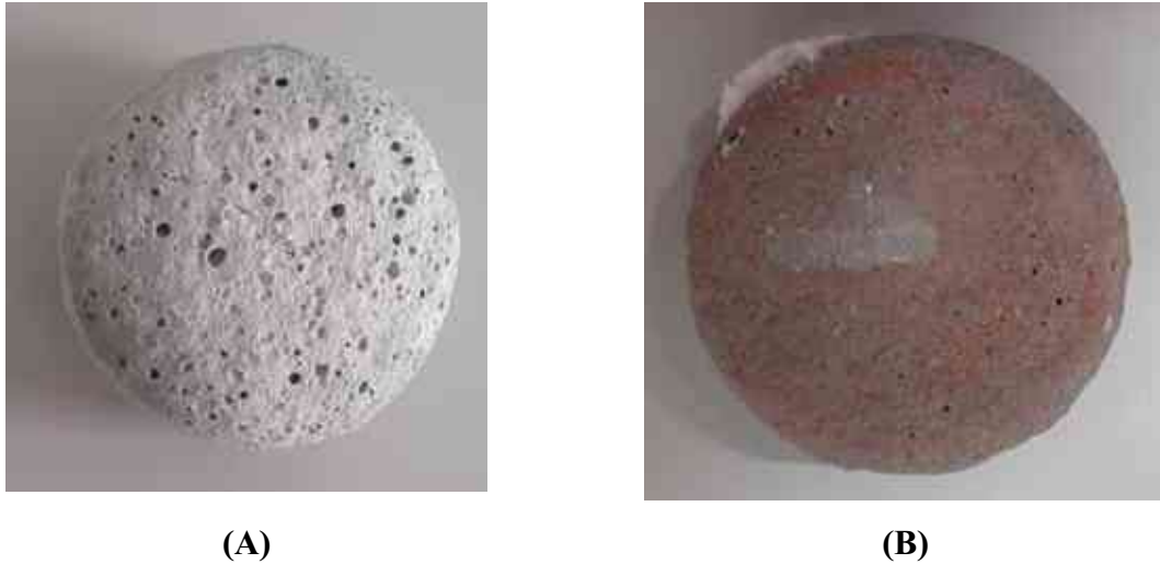
Figure 49. G20D53 sample in water - efflorescence (total dissolved salt) (A), Sample in acid - efflorescence (total dissolved salt) + oxidation (B)
