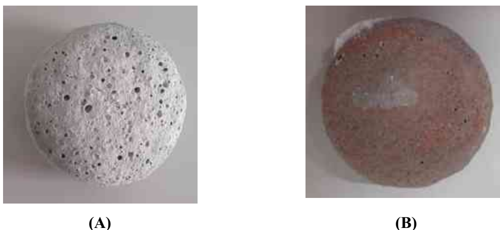
Figure C21. G20D53 sample in water - efflorescence (total dissolved salt) (A), Sample in acid - efflorescence (total dissolved salt) + oxidation (B)
