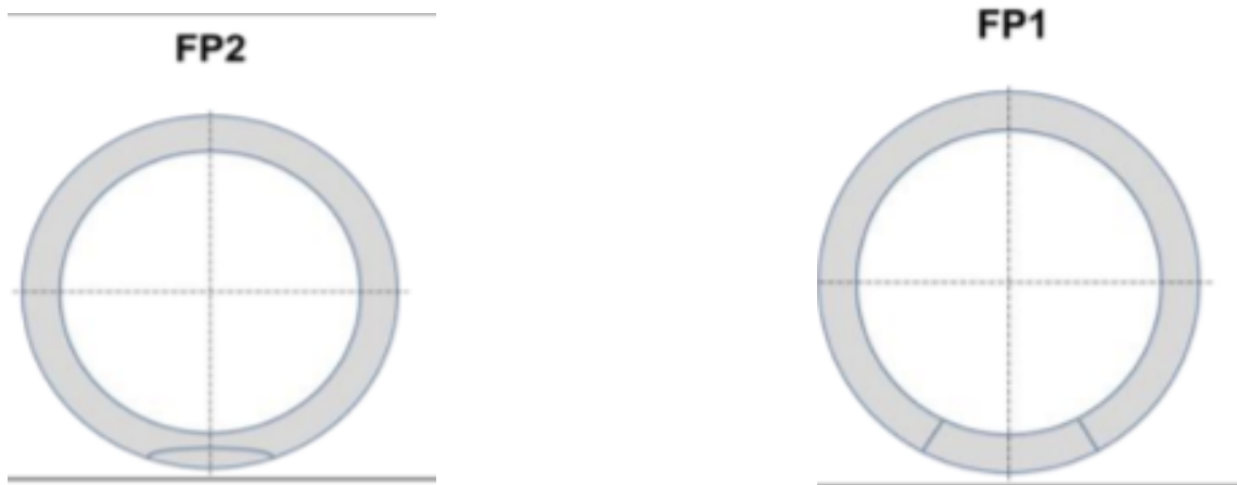
Figure 11. FP1, FP2 crack defect shapes
