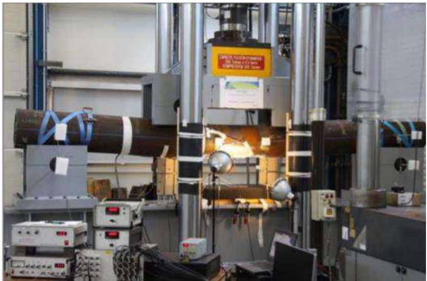
Figure 19 Four bending tests in reality [66]
