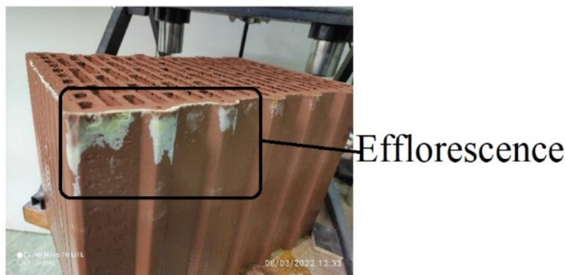
Figure 73. Efflorescence in masonry brick after immersing in water for a week followed by room temperature drying
