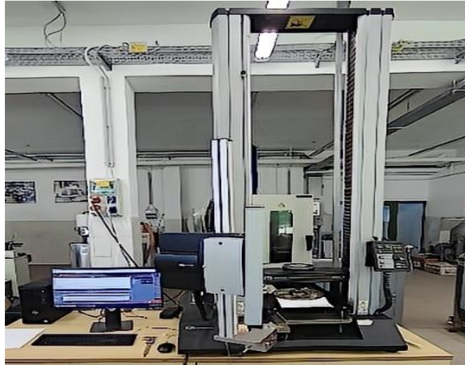
Figure 40. Hydraulic universal testing equipment
