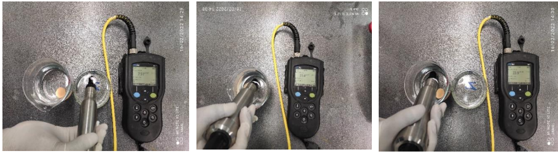
Figure 74. The TDS test for water after a week of immersing zeolite-poor rock-based bricks
