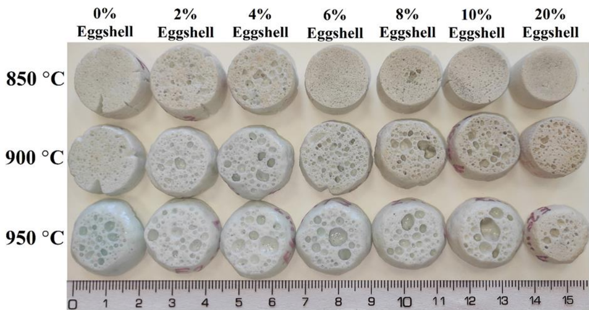
Figure 98. Photos of foamed samples with varied contents of eggshell sintered at different temperatures
