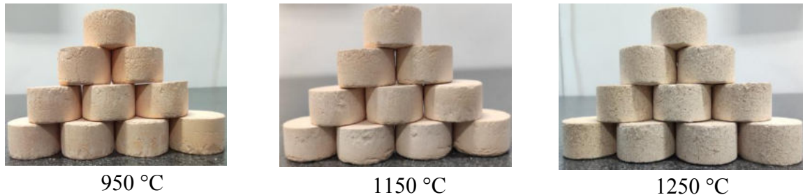
Figure 5. Laboratory-scale zeolite-poor rock/sawdust ceramic bricks sintered at different temperatures
