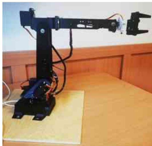
Figure 2.8 3D printed 6 DOF robot arm using PETG filament
