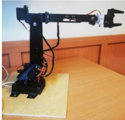
Figure 2.4 3D printed generation using PETG filament.
