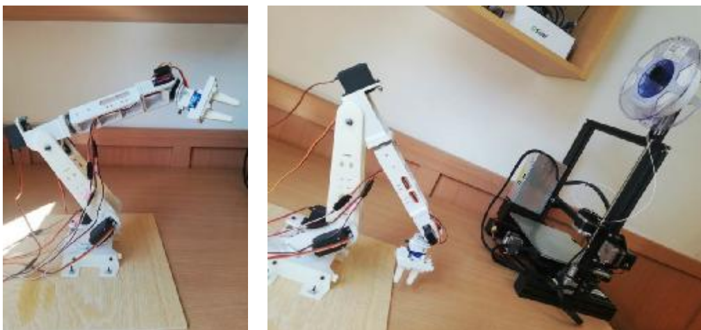
Figure 2.3 3D printed generation using PLA and ABS filament.
