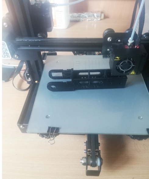
Figure 2.9 Printing operation for link 4 for the robot arm
