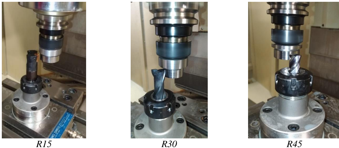
Figure 2.2. Cutting tools on the Force Measurement platform
