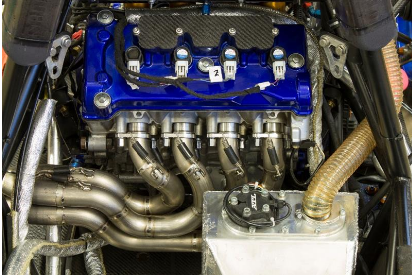
Figure 40 Honda CBR 600RR (PC 37) current engine exhaust manifold.
