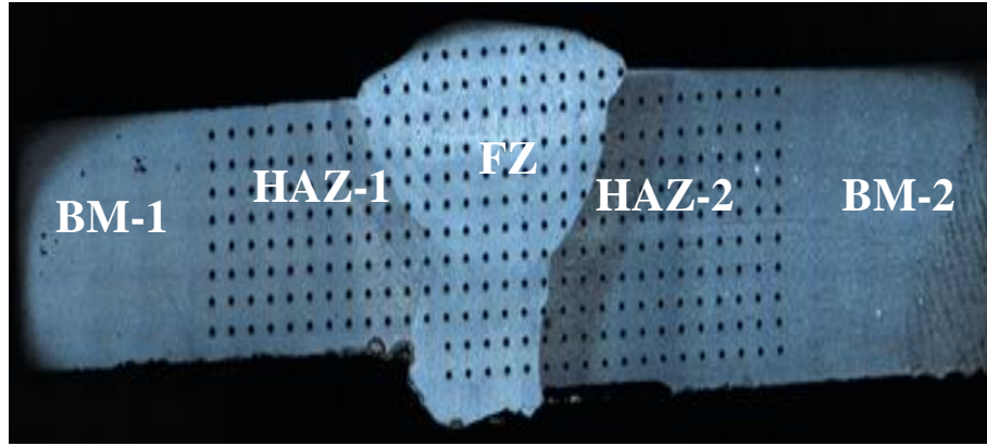
Figure 42. The specimen after hardness measurement
