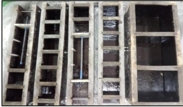
Figure 6.7 Molds were cleaned and oiled
