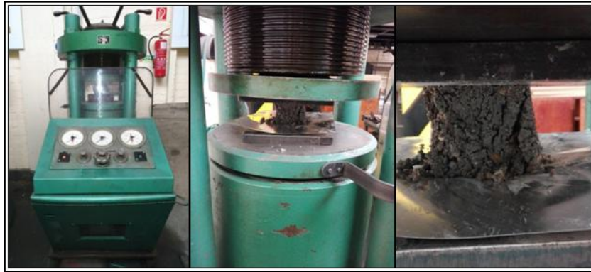
Figure 6.12 Machine of compressive strength during test the samples
