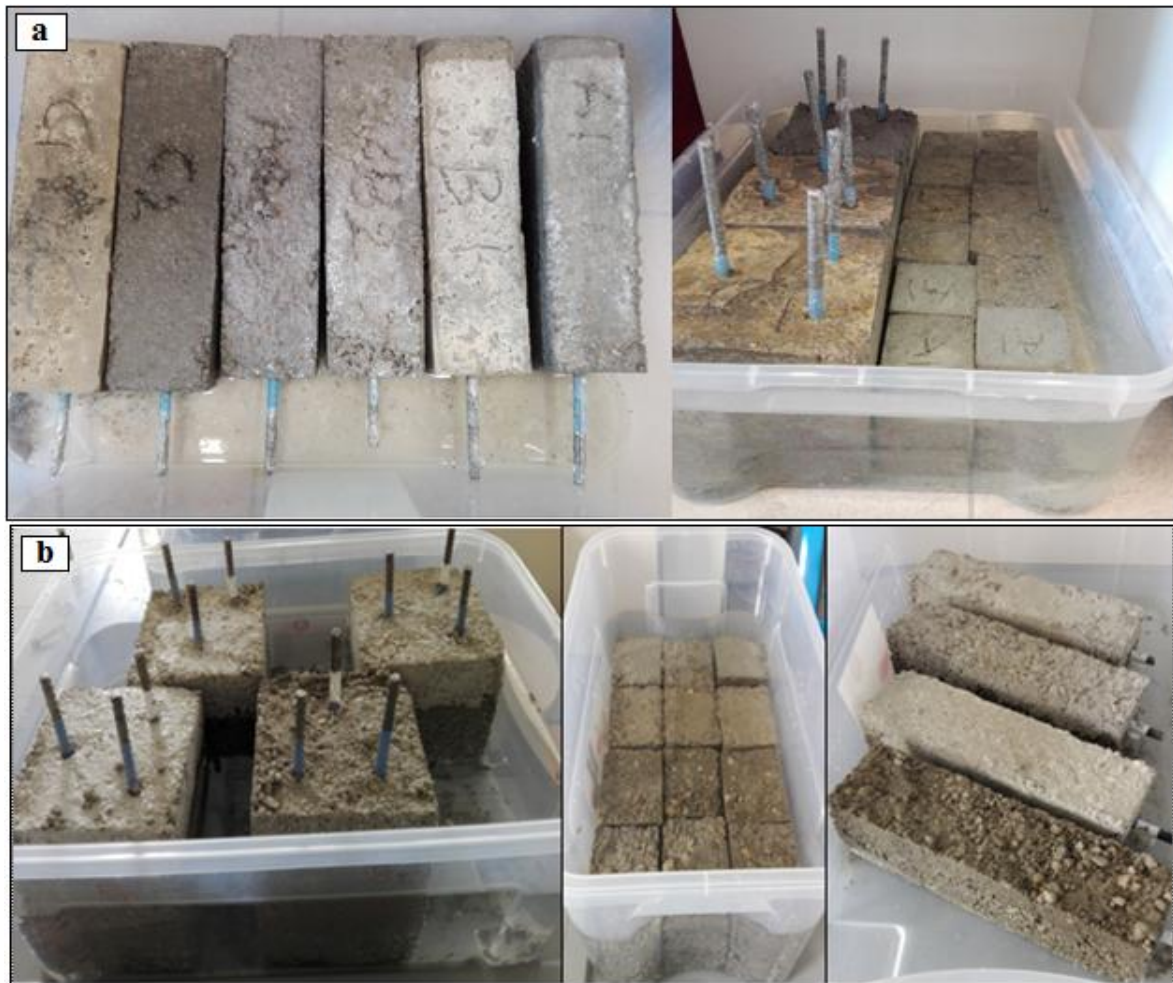
Figure 6.11 Specimens of half-cell corrosion potential test and linear polarization resistance test immersed partially and specimens of chloride ion ingress test completely immersed in 3.5% NaCl solution a) samples with green inhibitor, b) with calcium nitrate
