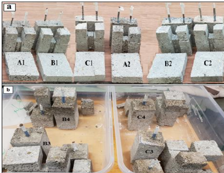
Figure 6.22 Reinforced concrete samples after cutting a) samples with green inhibitor, b) with calcium nitrate
