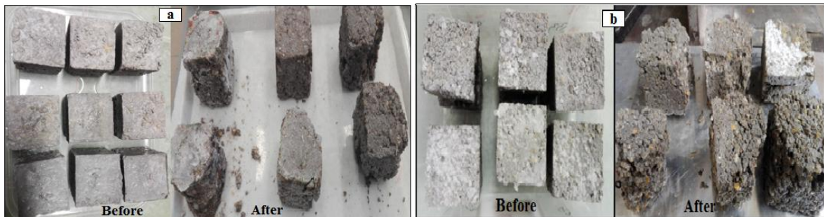
Figure 6.13 Specimens before and after compressive strength test a) samples with green inhibitor, b) with calcium nitrate
