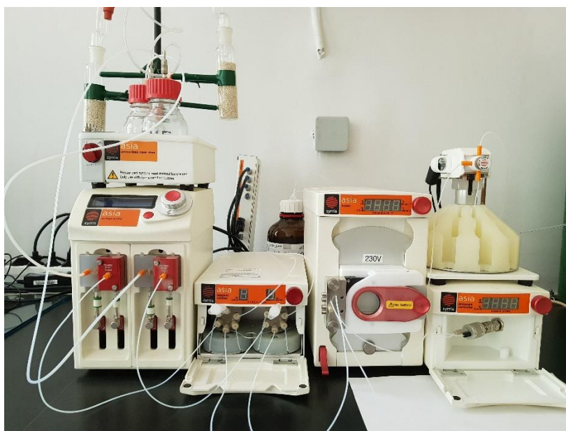
Figure 31: Microreactor setup: the Asia microflow system (Syrris Ltd., Royston, UK).
