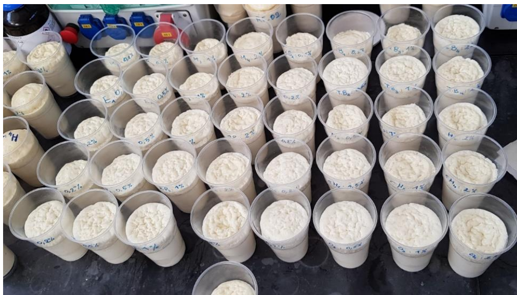
Figure 40: Flexible polyurethane foams, all with the concentration of monoalcohol in the range of 0.2, 0.5, 1.0, and 2.0%.
