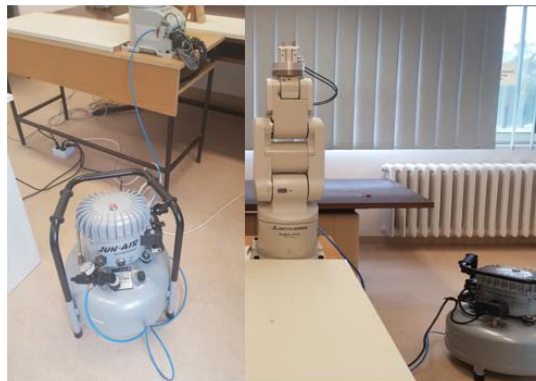
Figure 18. Connection between compressor and the gripper
