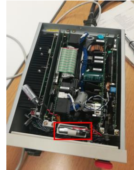
Figure 16. Changing the batteries of RV-2AJ arm Figure 17. Changing the batteries of controller
