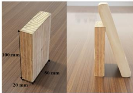
Figure 20. Measurement of support element
