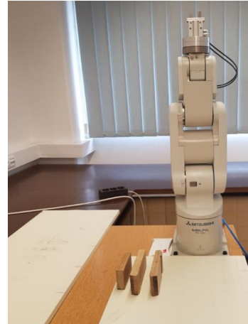
Figure 23. Pick and place scenario by RV-2AJ arm
