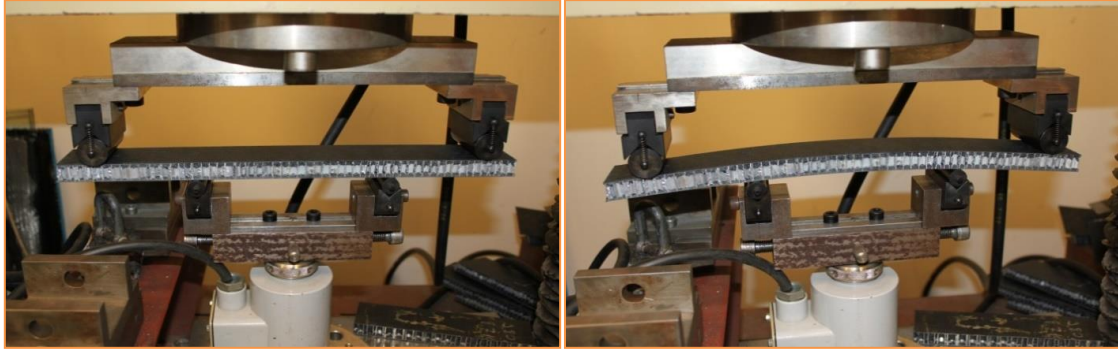
Figure 2: Experimental specimens (four-point bending test) for the sandwich panels consisting of aluminum honeycomb core and phenolic woven glass fiber face-sheet.
