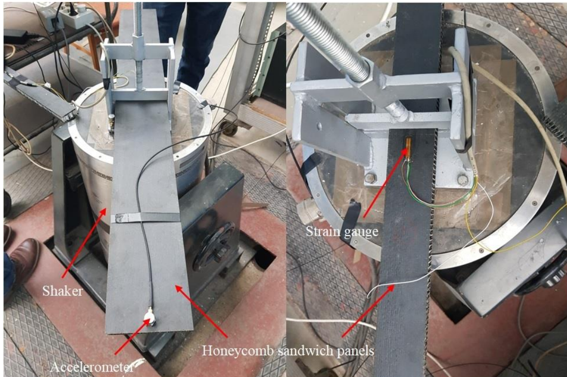
Figure 7: Experimental modal analysis (forced vibration test).
