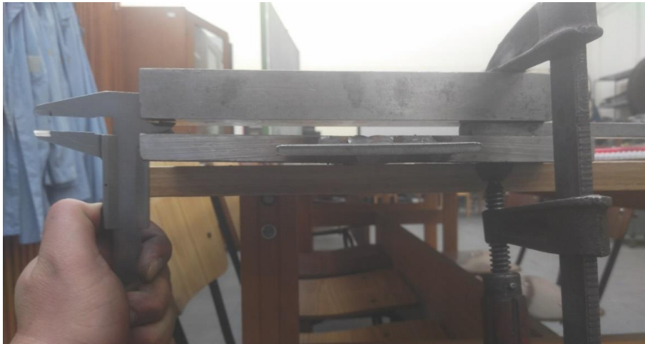
Fig. 5.2. Deformation scaling by vernier caliper.
