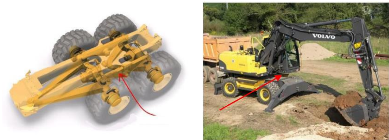
Fig. 2.14. Boggi beam (left) and excavator arm (right) [33].
