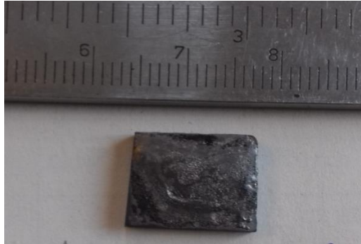
Figure C. Cast iron sample after the brazing process (Ni alloy foil+ iron coated NbC+Si powder without MA)
