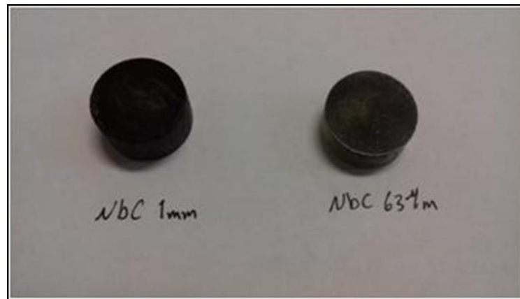
Figure 41. Iron coated NbC powder in resin samples
