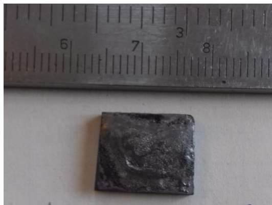
Figure 39. Cast iron sample after the brazing process (Ni alloy foil + iron coated NbC+Si powder without MA)
