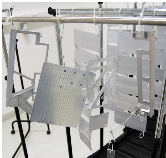
Figure 11. Ageing process for Zr4 based Cr3 coating over AA6082, Sentinel – 2 hardware
