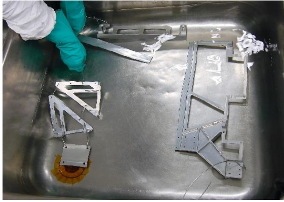
Figure 10. Post water immersion procedure for Zr4 based chromium conversion coated AA6082 sentinel-2 hardware's
