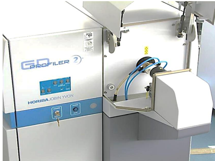
Figure 15. GD-OES device at University of Miskolc, Miskolc- Hungary
