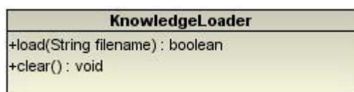
Figure 6.5. Knowledge loader class of Domain module
