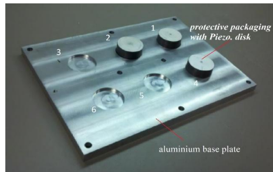
Figure 6. 4 The first layout Assembly design
