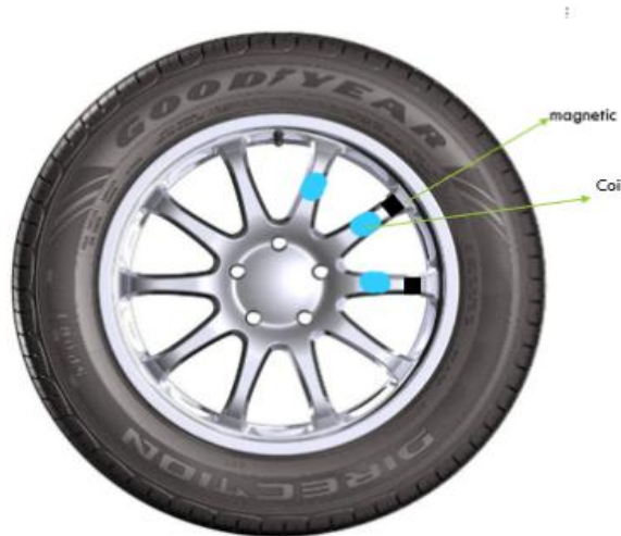
Figure 4. 4 The simple drawing about placement of magnetic and coil for AD case
