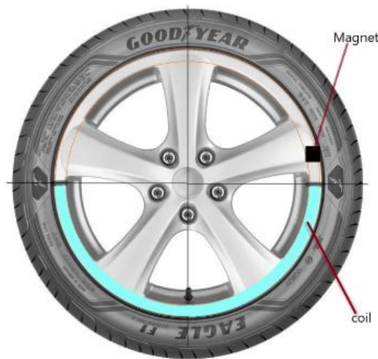
Figure 4. 1 The simple drawing about placement of magnetic and coil for RD case
