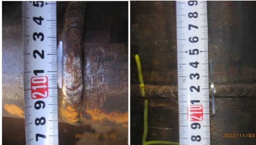
Figure 16 Artificial notch in the girth weld HAZ of the Y10 pipeline section (left), artificial notch through the girth weld of the Y8 pipeline section (right)
