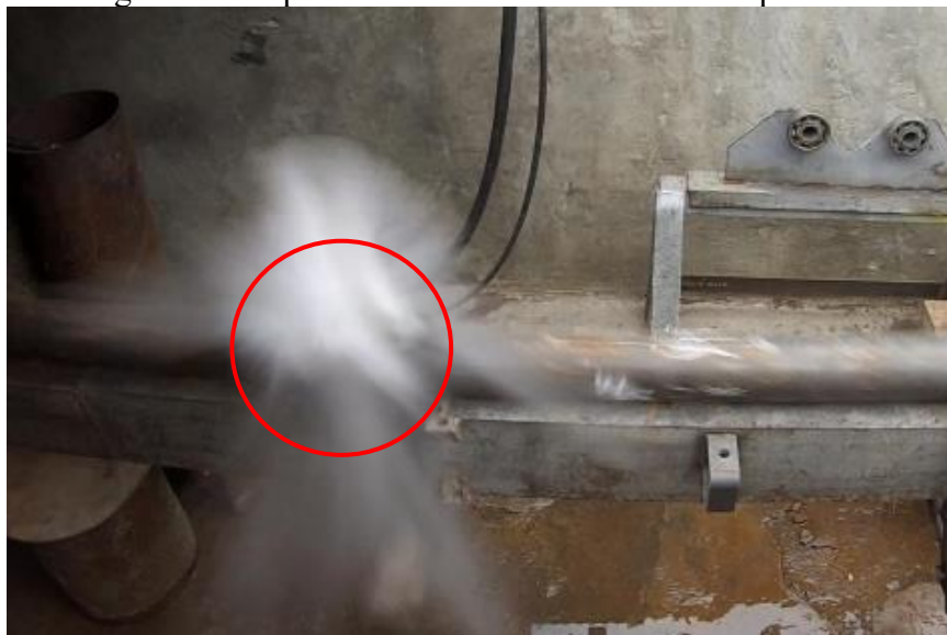
Figure 22 Y1 pipeline section at the moment of its failures
