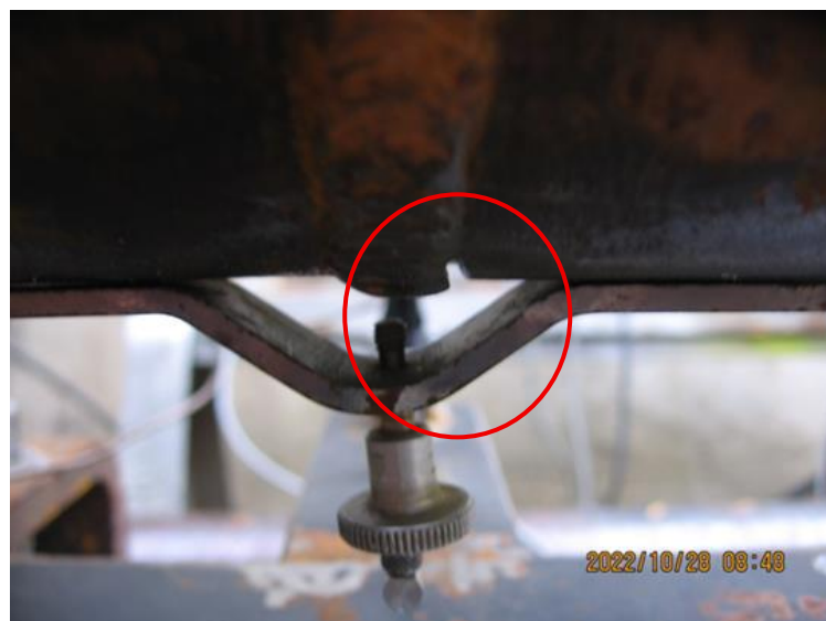
Figure 15 The artificial notch configurations
