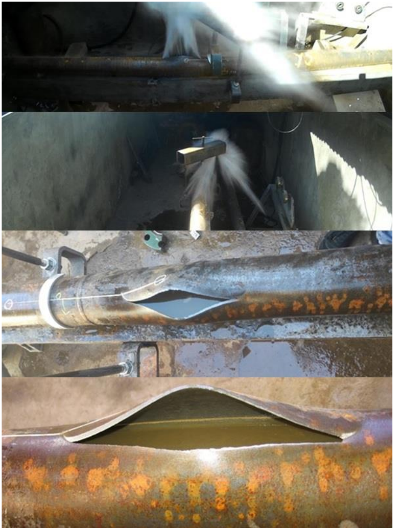
Figure 87 Pipeline section Y5 after the burst test: pipe section displaced on the support beam in the test pit (top), damaged section (second), moment of failure of the pipeline section Y6 during the burst test: side view (third), longitudinal view (bottom)
