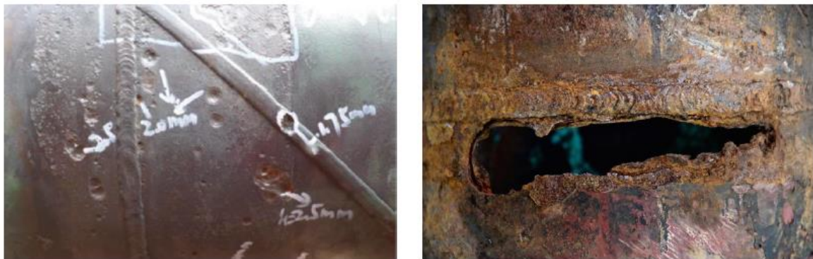
Figure 30 Corrosion defects near and on pipeline welded joints [59], [60]
