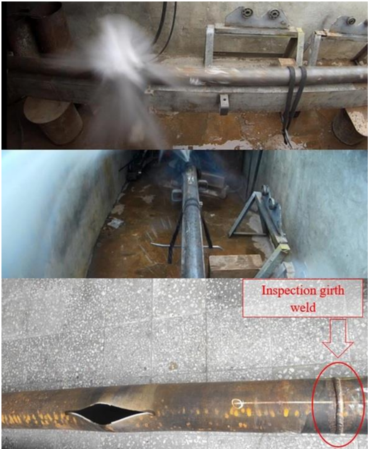
Figure 83 Moment of failure of the pipeline section Y1 during the burst test: side view (top), longitudinal view (middle), the Y1 pipeline section after the burst test: the damaged section and the tested girth weld (bottom)
