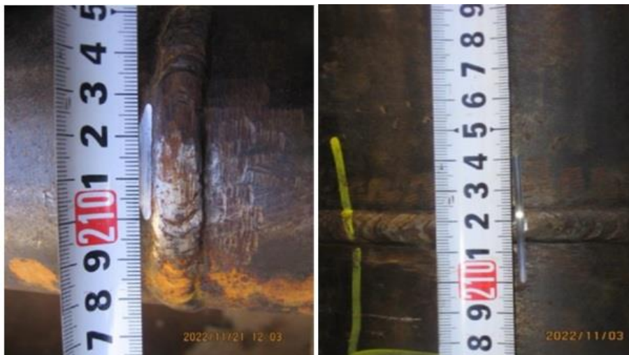
Figure 66 Artificial notch in the girth weld HAZ of the Y10 pipeline section (left), artificial notch through the girth weld of the Y8 pipeline section (right)
