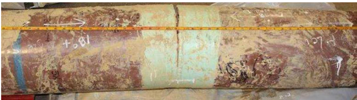
Figure 27 Girth weld crack caused by different pipe and ditch profiles [56]
