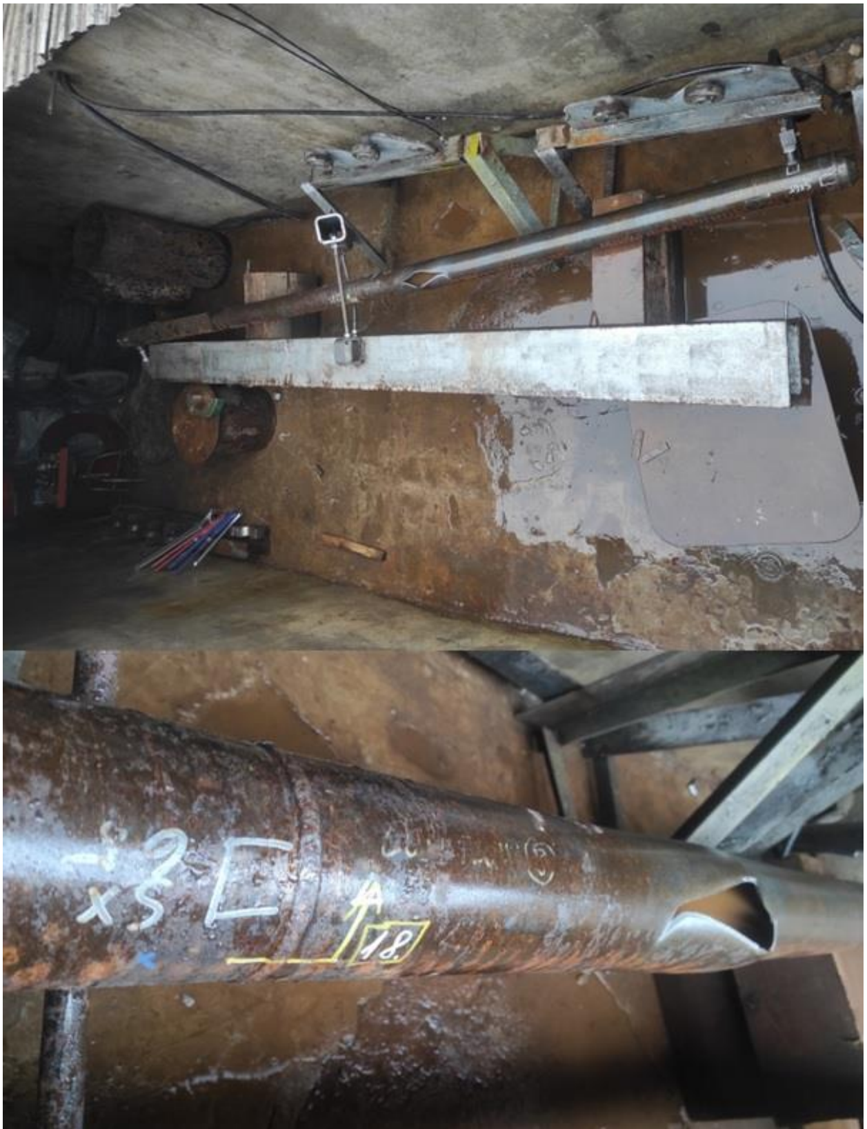
Figure 88 Pipeline section Y6 after burst test: section of pipe (with the burst support beam and the damaged external load transfer device) in the test pit (top), damaged section (bottom)
