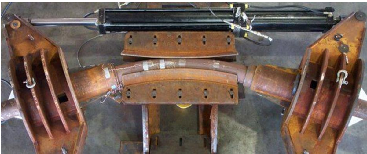
Figure 38 Test setup for an experimental pipe section subjected to or capable of complex loading conditions [79]
