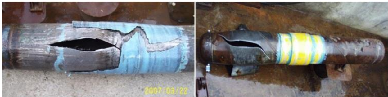
Figure 34 Pipeline sections after fatigue and burst test with reinforced girth weld; left: system developed at University of Miskolc; right: Clock Spring repair system [66]
