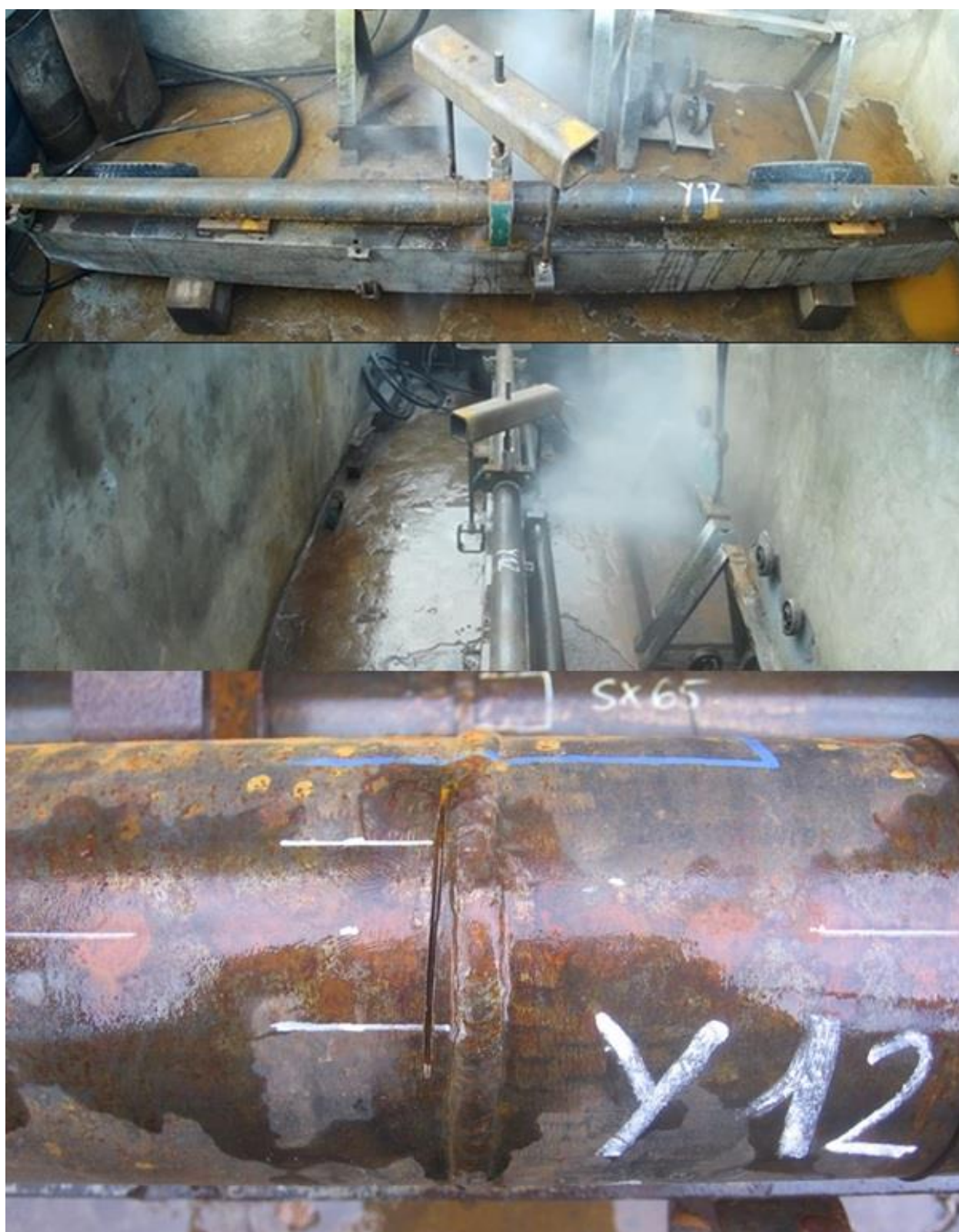
Figure 94 Moment of failure of the Y12 pipeline section during the burst test: side camera image (top), longitudinal camera image (middle), tested pipe section Y12 after the burst test: the damaged section (bottom)
