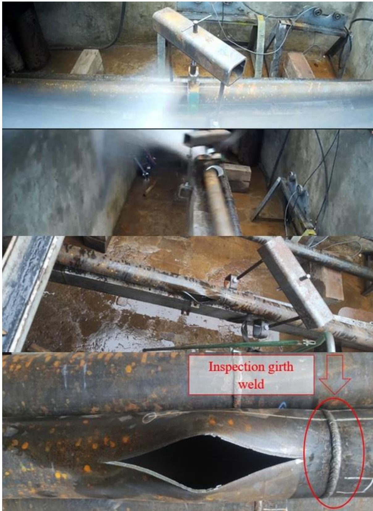
Figure 89 Moment of failure of the pipeline section Y7 during the burst test: side view (top), longitudinal view (second), the pipeline section Y7 after failure: the pipeline section displaced on the supporting beam (and the damaged external load transfer structure) in the test pit (third), the damaged section (bottom)
