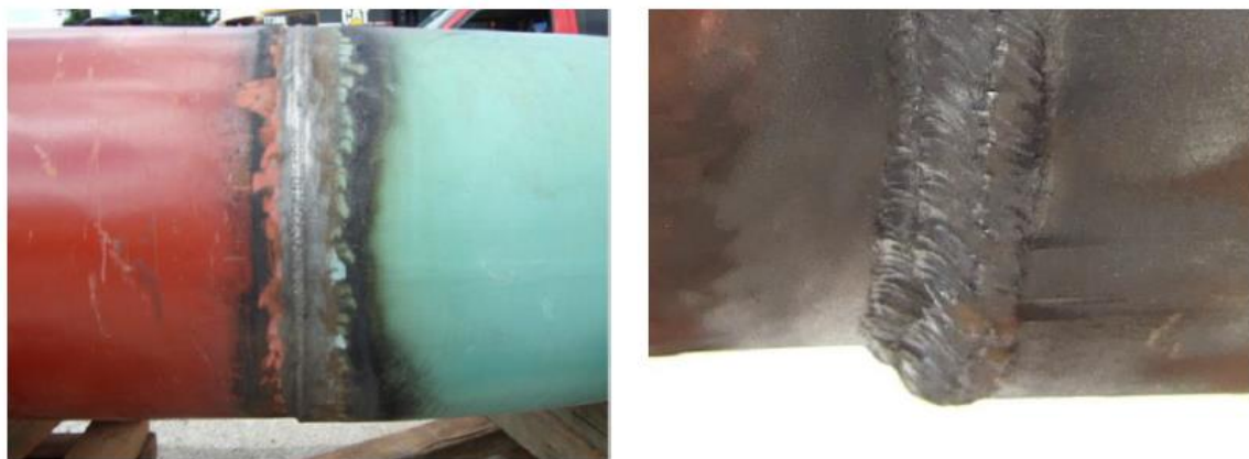
Figure 25 Unacceptable treatment of an axial misalignment [54], [55]
