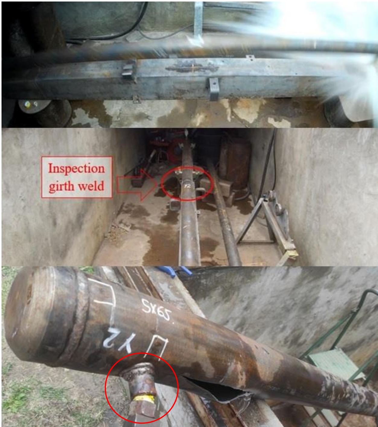
Figure 84 Moment of failure of the pipeline section Y2 during the burst test: side view (top), longitudinal view (middle), the pipeline section Y2 after the burst test: the pipeline section with the damaged section (and the damaged coupling fitting highlighted with red circle) partially ejected from the test pit (bottom)
