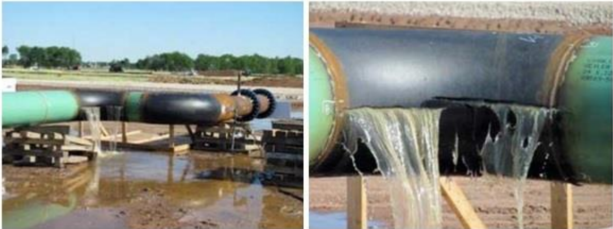
Figure 42 Catastrophic failure of a pipe arch section during a pressure test [102]
