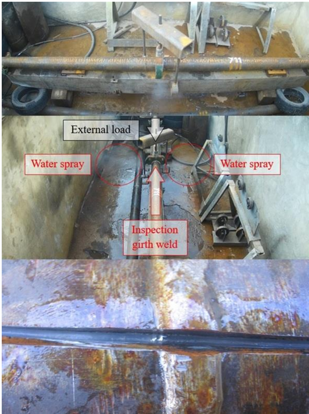
Figure 93 Moment of failure of the Y11 pipeline section during the burst test: side camera image (top), longitudinal camera image (middle), the pipeline section Y11 after the burst test: the damaged section (bottom)
