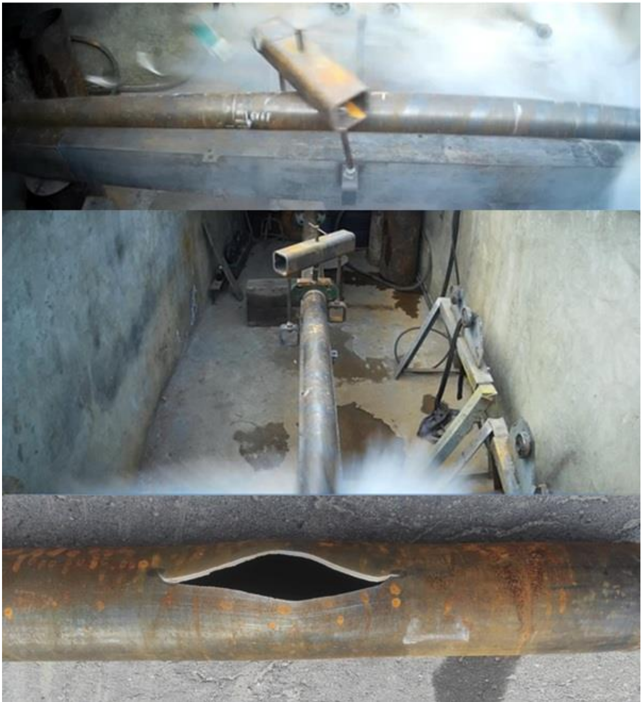
Figure 85 Moment of failure of the pipeline section Y4 during the burst test: side view (top), longitudinal view (middle), the pipeline section Y4 after the burst test: the damaged section (bottom)
