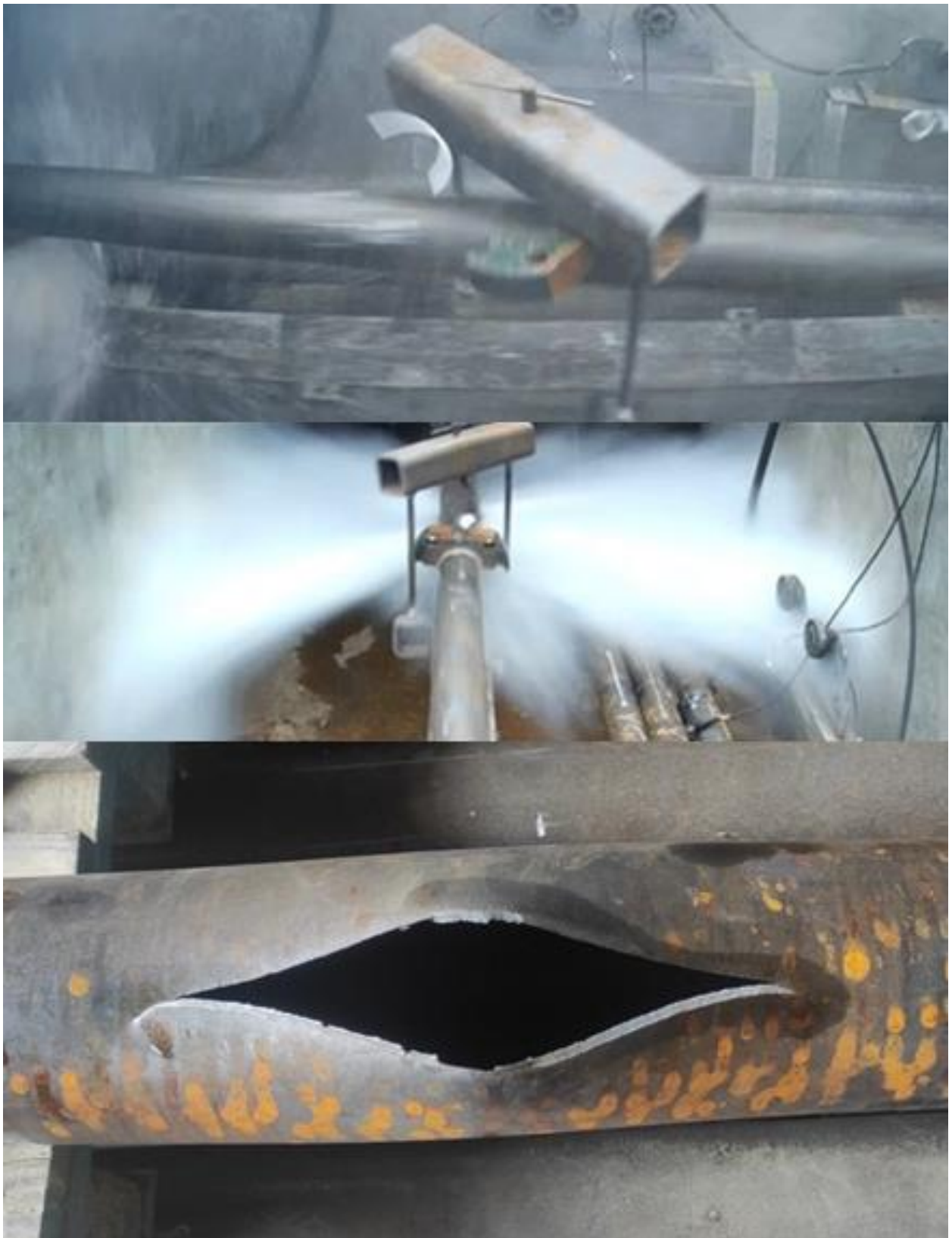
Figure 92 Moment of failure of the pipeline section Y10 during the burst test: side view (top), longitudinal view (middle), the pipeline section Y10 after the burst test: the damaged section (bottom)
