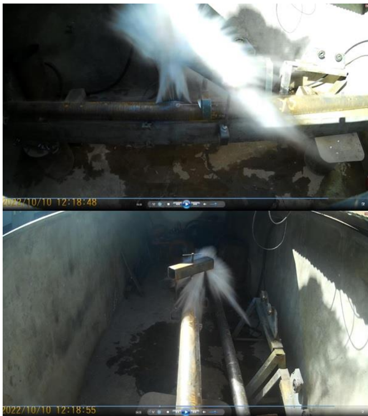
Figure 86 Moment of failure of the pipeline section Y5 during the burst test: side view (top), longitudinal view (bottom)
