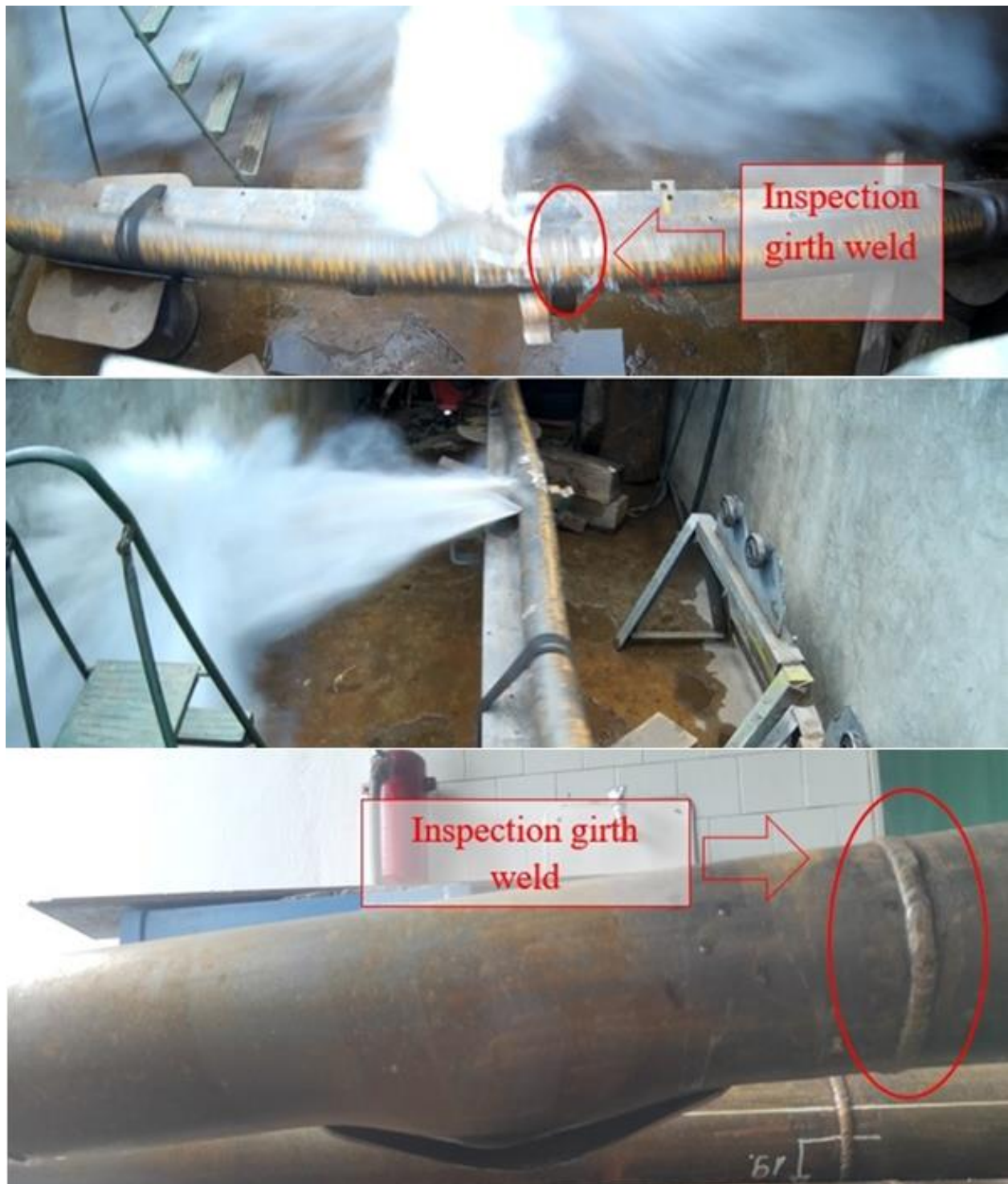
Figure 82 Moment of failure of the pipeline section Y3 during the burst test: side view (top), longitudinal view (middle), the Y3 pipeline section after the burst test: the damaged section and the tested girth weld (bottom)
