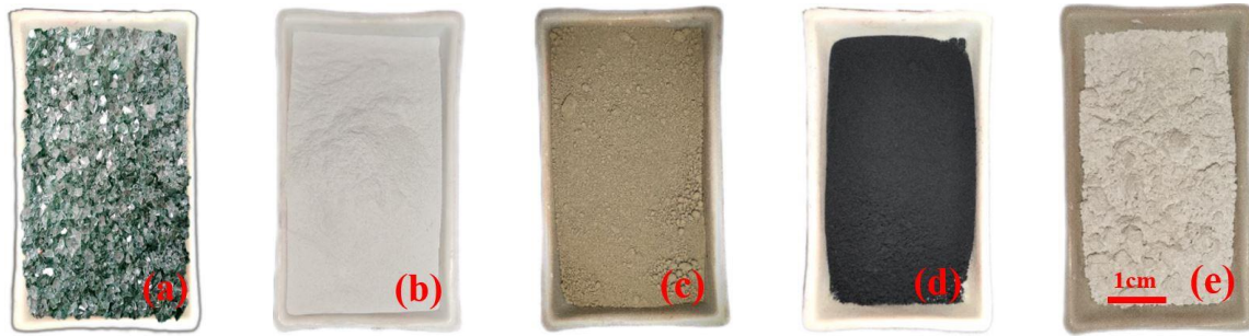
Figure 1. foam glass raw material a) Waste glass particles, b) virgin glass powder, c) SiC, d) Soot, e) Al 2 O 3 , photos are taken by mobile phone camera (iPhone 13 pro max).
