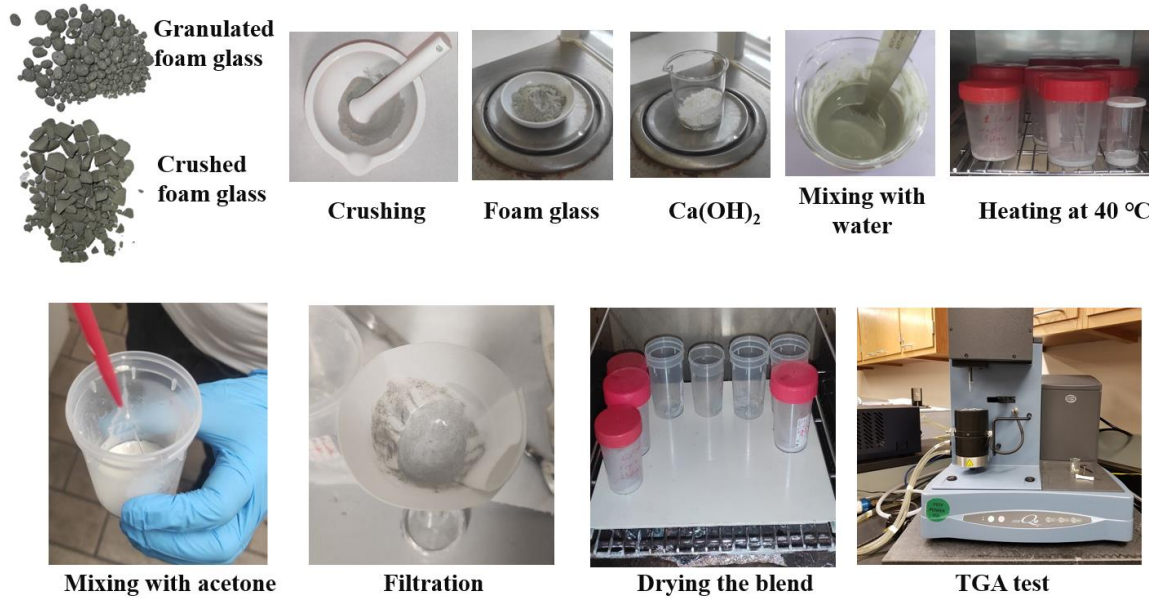
Figure 4. The procedure of testing ASR using a TGA device
