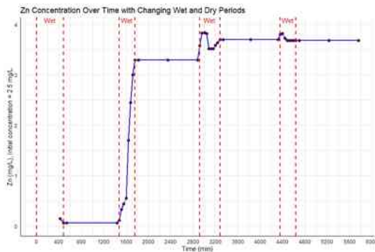
Figure 4-30 Breakthrough curve of \text{Zn}^{2+} concentration performance in the sand column of the SAT system during wet and dry periods
