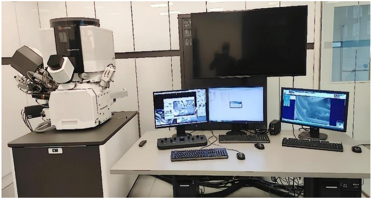
Figure 8. Helios G4 PFIB CXe DualBeam SEM setup in University of Miskolc
