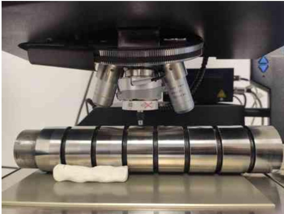
Figure 12. Measuring microhardness (HV 0.2)
