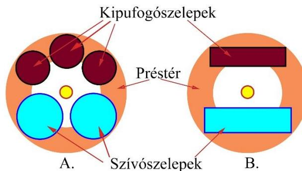
Figure 3: Comparison of the size of the squish area in the cylinder head of the engine with a poppet valve (A) and the engine with a swinging valve (B) (the yellow circle indicates the spark plug).
