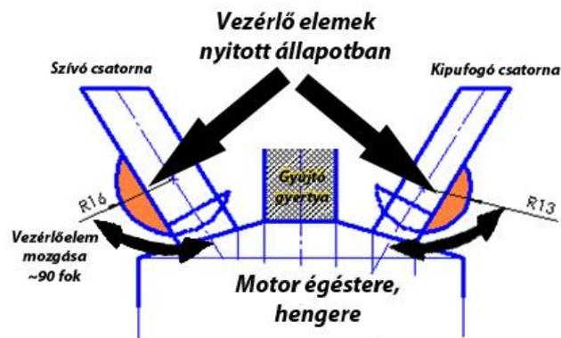
Figure 2: Schematic design of a swinging valve system
