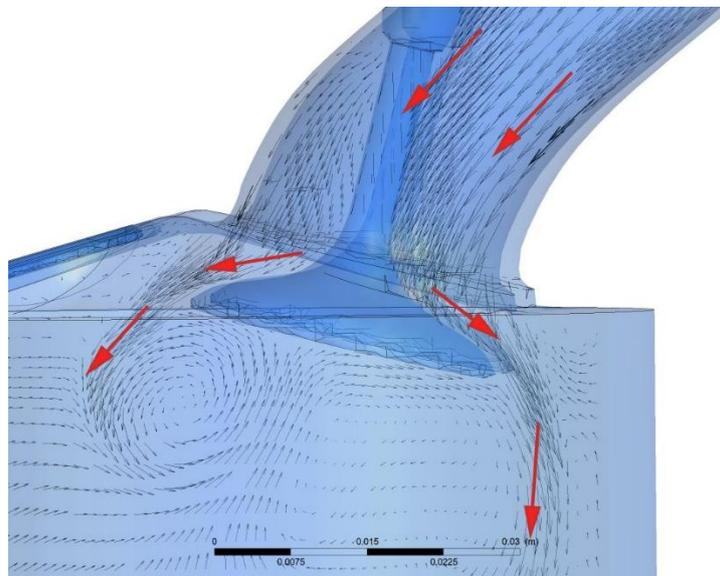
Figure 1: Flow deflecting behaviour of the valve head
