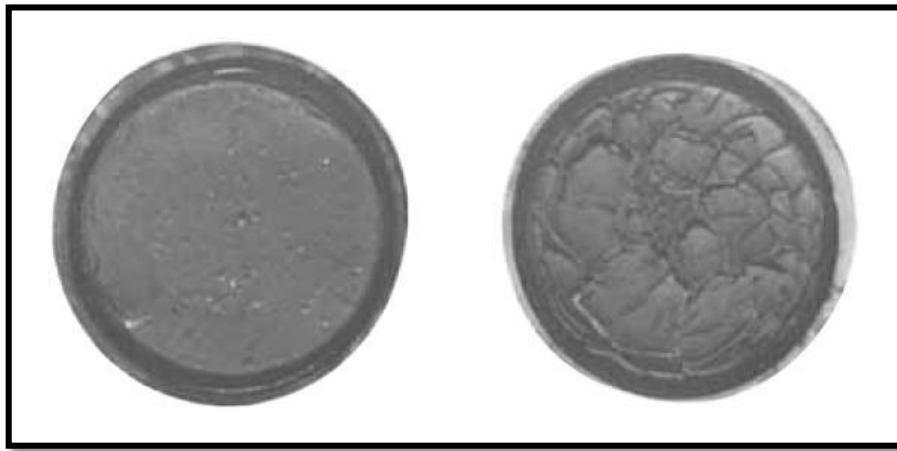
Figure 8: Cracking effect of filter cike using oil only (left) and Pipe-Lax-oil mixture (right) ( Drilling Fluids Engineering Manual 2007 )
