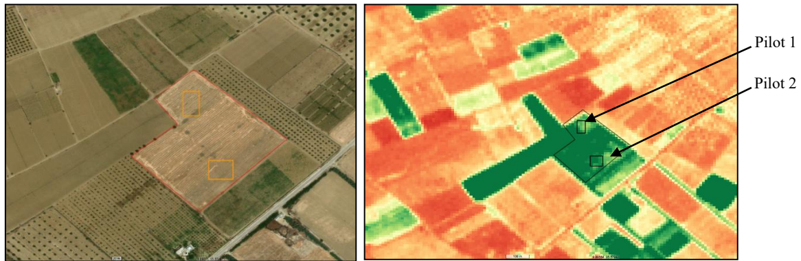
Figure 15. True-Color Imagery (Left) and NDVI (Right) for Pilot Sites 1 and 2
