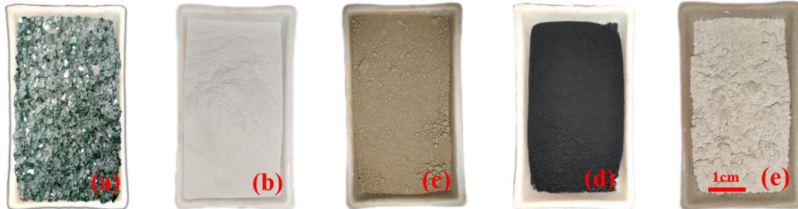
Figure 13. foam glass raw material a) Waste glass particles, b) virgin glass powder, c) SiC, d) Soot, e) Al 2 O 3 , photos are taken by mobile phone camera (iphone 13 pro max)
