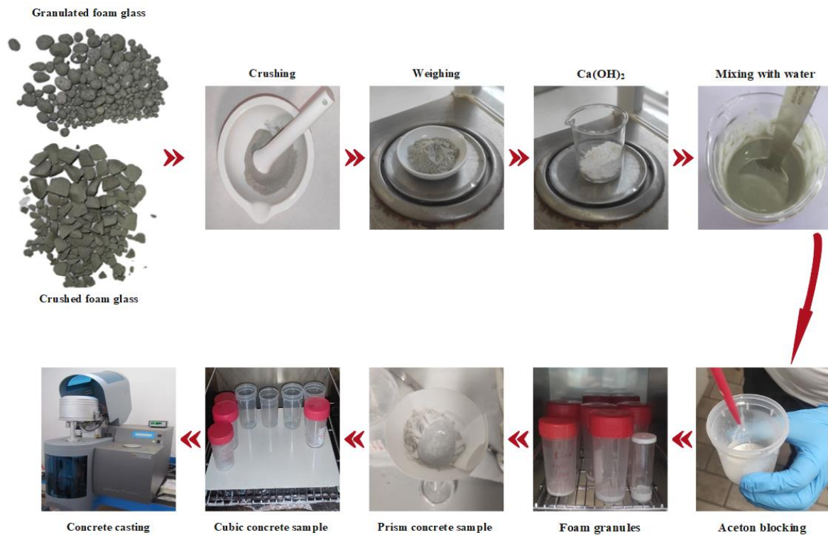
Figure 21. The procedure of testing ASR using a TGA device
