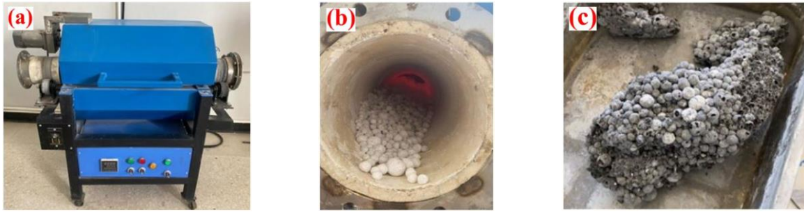
Figure 7. Fabrication process of granular foam glass aggregates, a) electric rotary furnace, b) rotation in alumina tube, and c) foam glass granules processed at 900°C [144]
