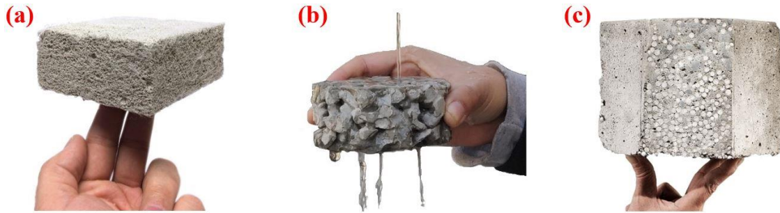
Figure 1. Three typical types of lightweight concretes. a) foamed concrete [9], b) no-fine concrete [10], and c) lightweight aggregate concrete [11]
