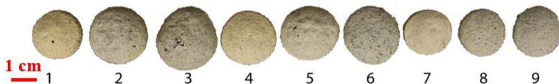
Figure 47. Nine groups of foam glass specimens – the compositions are according to Table 4. Sintered at 842 °C, heating rate of 5 °C/min, and holding time of 10 min
