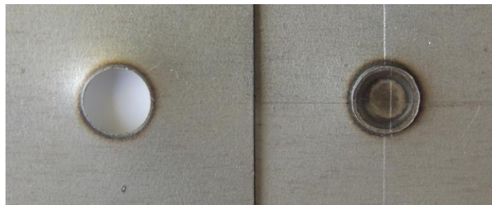
Figure 7.5. Plug failure mode in sample C1 of MS1400.
