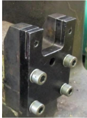
Figure 10.4. The new RSW specimen's holder [71].
