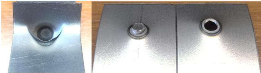
Figure 7.8. The failure mode in sample T1(plug-in base metal) is on the left and the failure mode in sample T3 (Plug) is on the right in DP600 samples.
