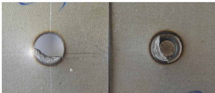
Figure 7.6. Partial plug failure mode in sample C3 of MS1400.
