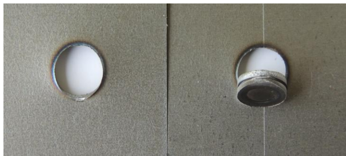
Figure 7.9. Plug failure mode in sample T10 of T-S test samples.
