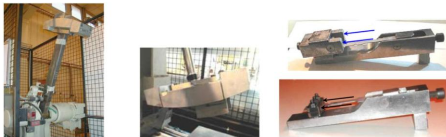
Figure 3.13. The redesigned hammer and specimen holder [158]
