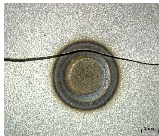
Figure 9.6. Top view of eyebrow shape crack propagation in MS1400 steel
