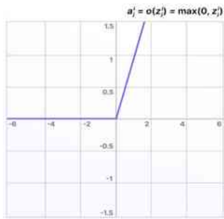
Figure 20. ReLU Activation Function (Source: www.encord.com )
